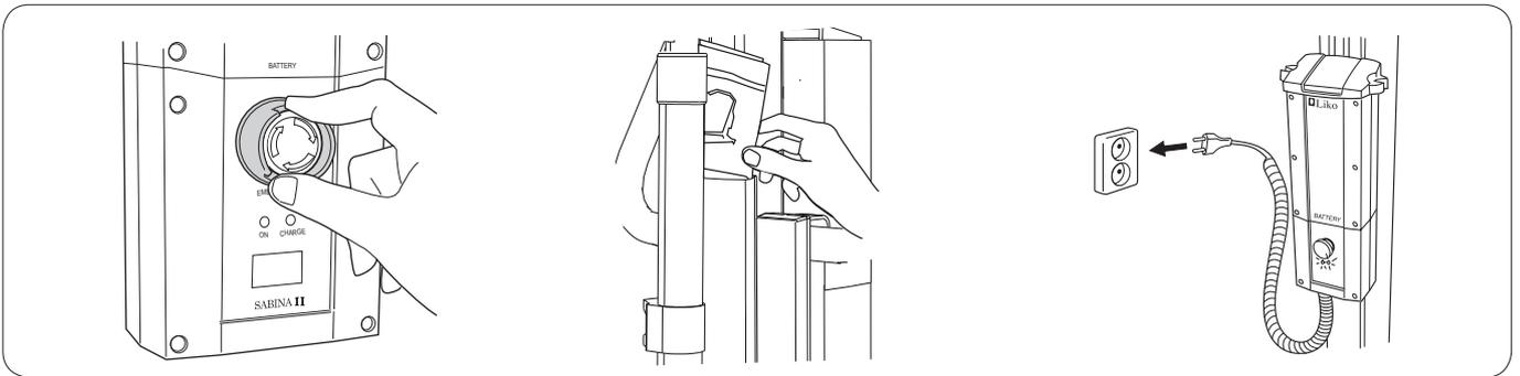
10. Release the emergency stop by turning the button in the direction indicated by the arrows on the button.
