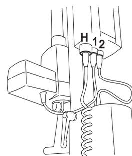
3. A) Remove the locking handle from the lift arm. Slide the sling bar onto the lift arm with the opening on the lifting hooks facing forward (see illustration).
