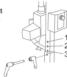
1. Remove the locking handle from the base. Place the lift mast in the foot of the base.
