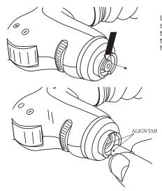
Use your fingernail or a small prying instrument to remove the lamp from the ophthalmoscope head base.
