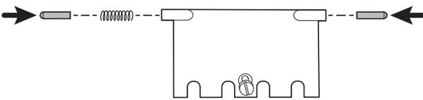
Insert a spring and two pins into the communications door as shown.
