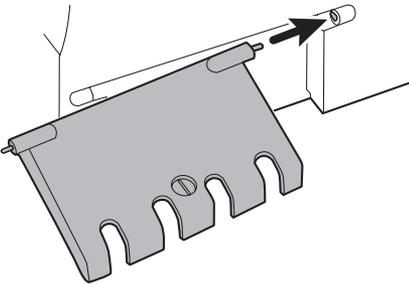
With the bottom of the housing on the antistatic mat, insert the pin on the right side of the door into the hinge of the rear housing.
