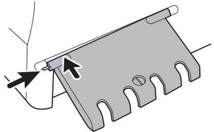
Press the pin into the left side of the door and slide the door into the hinge of the rear housing until it snaps into place.
