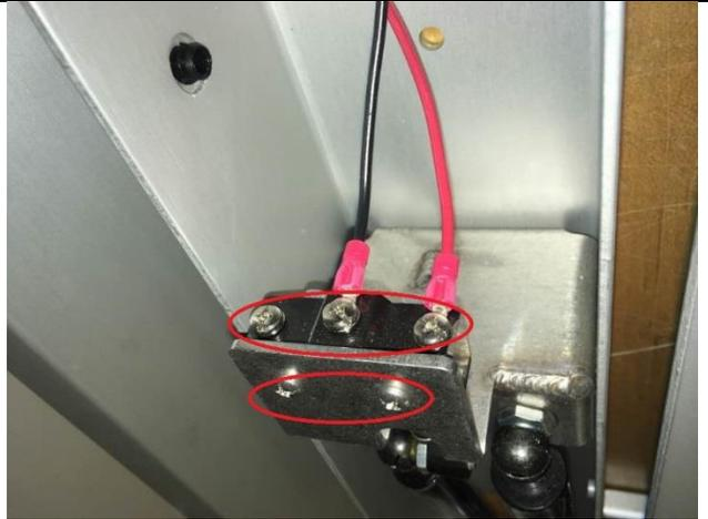
9. Use a 1/8" Allen wrench to remove the deck cover's screws
