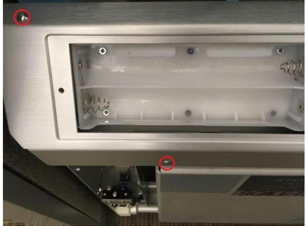
14. Use a small Philips screwdriver to remove the screws on battery holder
