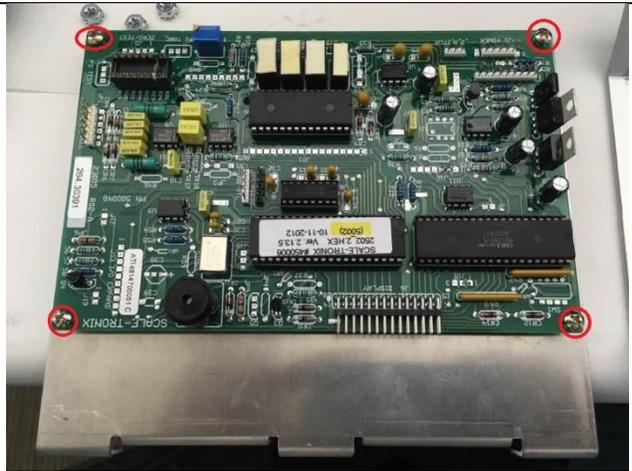
12. Use a #1 Phillip screwdriver to remove the screws on the display board
