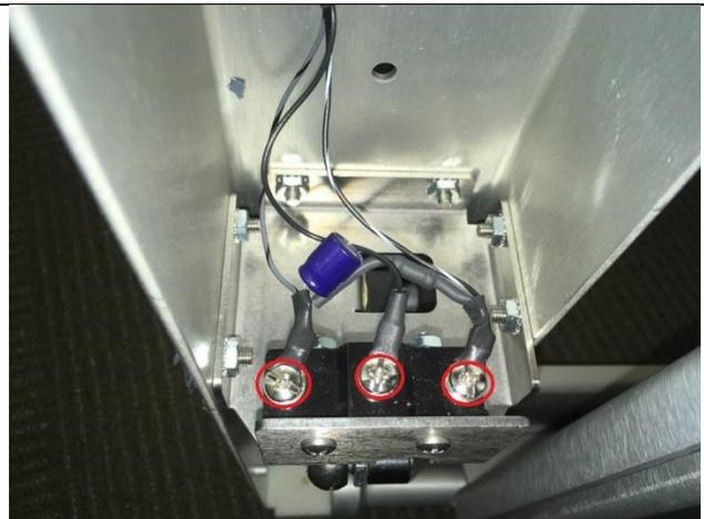
17. Use a #1 Phillip screwdriver to remove the bracket mount's screws
