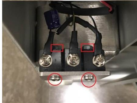
20. Use a 3/8" wrench to remove the nuts on the mounting bracket
