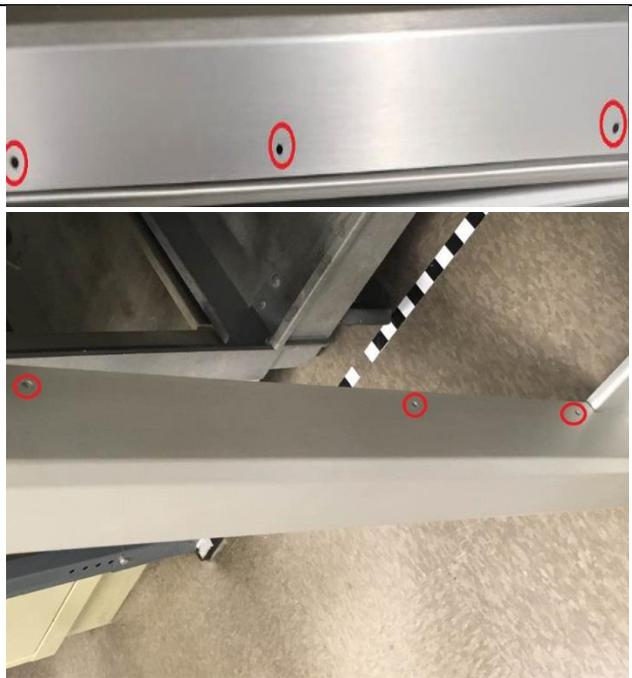
6. Use a 3/8" wrench to remove the nuts on the mounting bracket
