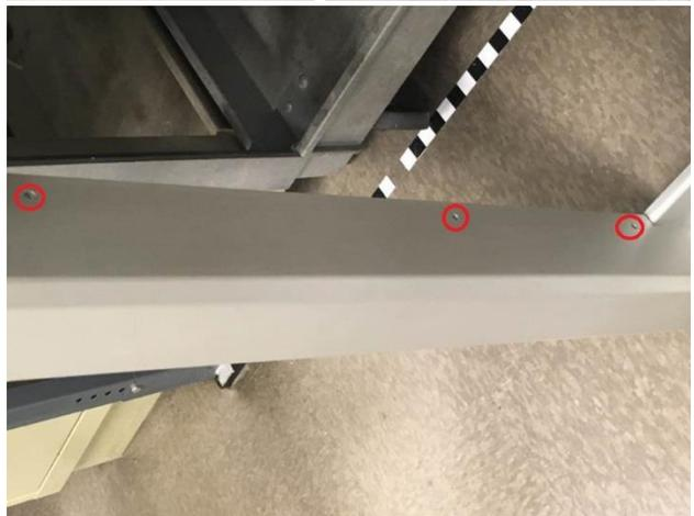
19. Use a #1 Phillip screwdriver to remove the bracket mount's screws
