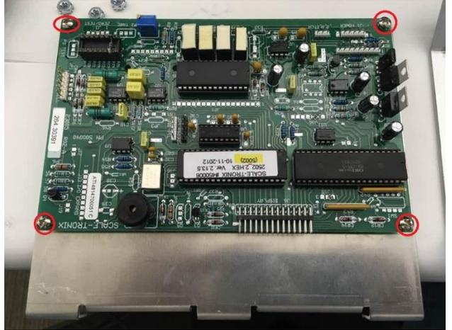
11. Use a #1 Phillip screwdriver to remove the screws on the display board
