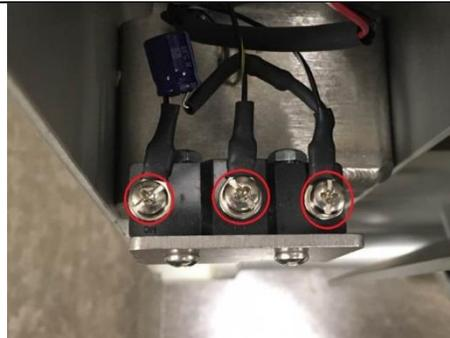
Use a 3/8" wrench to remove the nuts
