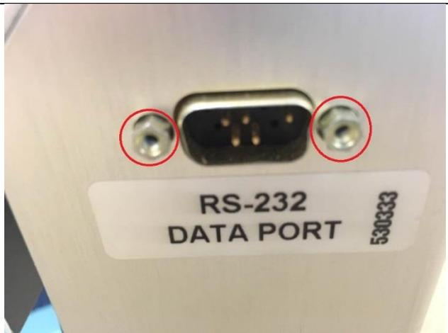
23. Use a 1/8" Allen wrench to remove the screws on the deck cover
