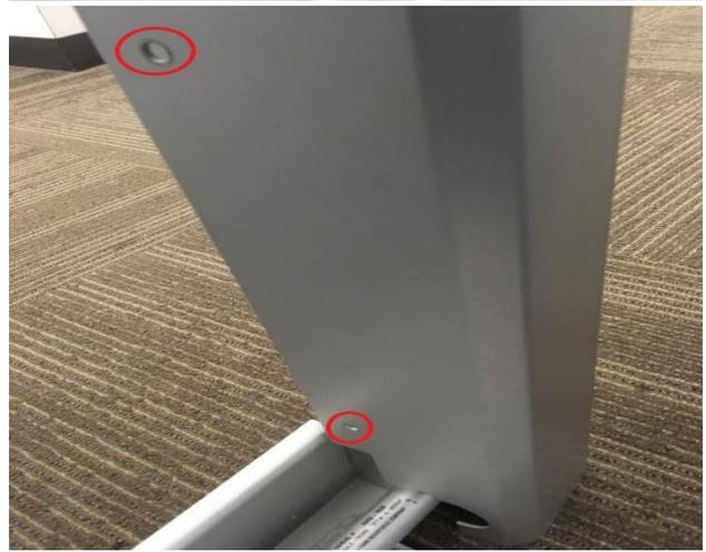
16. Use a #1 Phillip screwdriver to remove screws on the momentary switch
