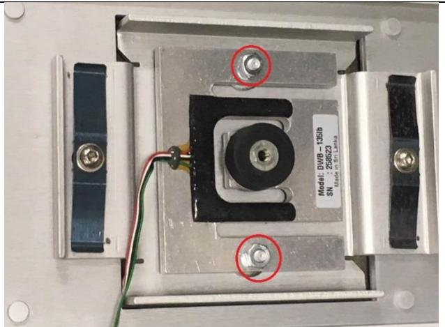
13. Use a 1/8" Allen wrench to remove the screws on the springs and the rubber isolator
