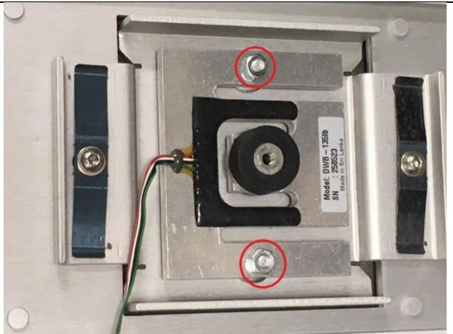
35. Use a 1/8" Allen wrench to remove the screws on the springs and the rubber isolator
