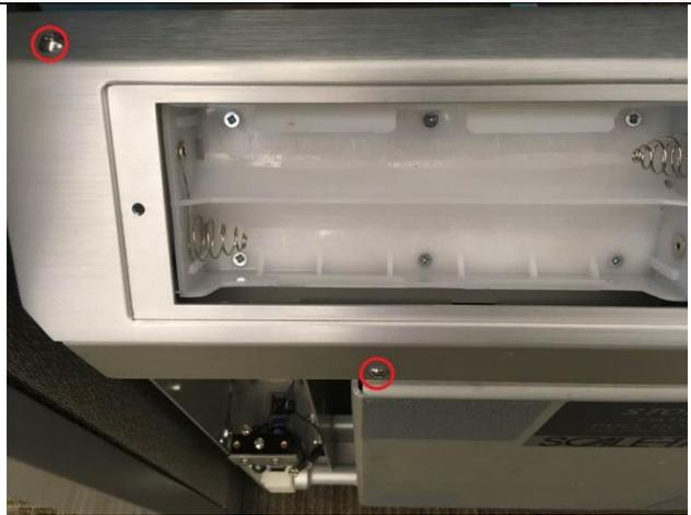
15. Use a small Philips screwdriver to remove the screws on the battery holder
