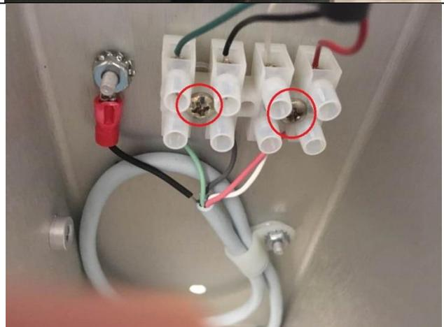
20. Use a 5/16" socket to remove the screws on the wire with loop and the cable clamp
