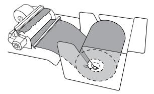
6. Pull the paper under the print head lever and push the green knob down to push the print head lever down.
