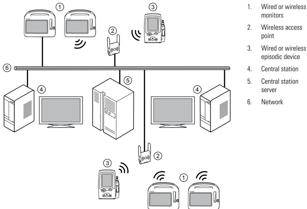
In this configuration, one or more central stations are connected to a single Connex server. The central stations share common data, such as configuration data, user definitions, and patient information by maintaining it on the Connex server.
