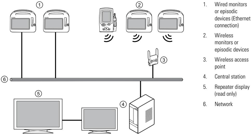
In this configuration, continuous and episodic devices communicate over the network to the central station. The central station contains all the software needed to monitor patients' continuous parameters and episodic data on a single computer.
