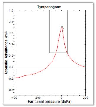
The tympanogram is plotted with the normative data box and the peak indicated by the X placed on the curve. Any adjustment of the peak is performed on the instrument and cannot be changed in TympView program.
