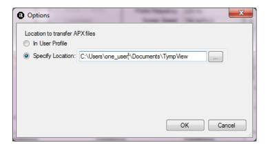
The specific location may be typed directly into the text box or the button at the end of the text box may be selected to browse the PC to select the directory.
