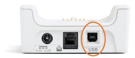
The MicroTymp 4 unit must be placed in the cradle for data to be transferred. The cradle must be plugged into power and the device should be turned on. The transfer of data is initiated from the TympView program running on the PC.
