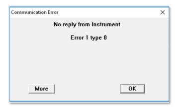
This message is displayed when the download from the Tympanometer is selected and the device is not turned on. Confirm that the device is turned on and the cradle is plugged into power.
