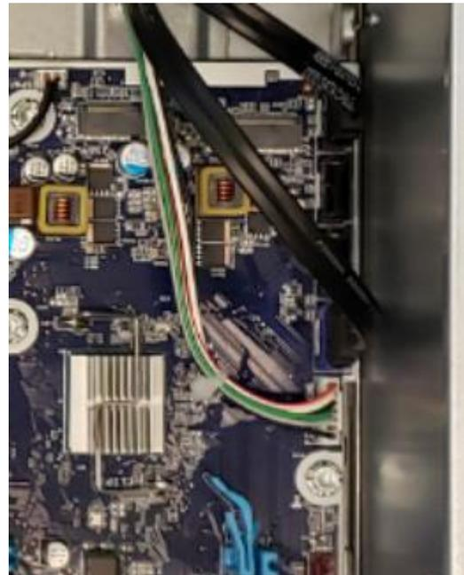
**NOTE:** When replacing the system board, be sure that the CPU cooler and system memory are removed from the defective motherboard and installed on the replacement motherboard.
