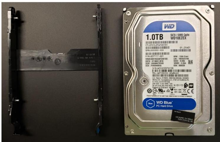
Once the rails are in place, slide the new drive into the drive rack, and reinstall the data and power cables.
