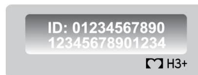
To end recording early, the battery may be removed from the recorder to stop recording. Reinsertion of the battery will display the ID in reversed color as shown above.
