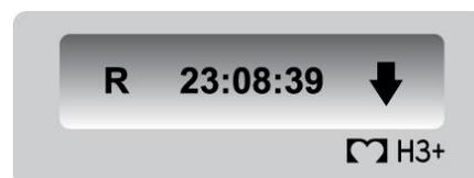
To enter an event after the first minute of recording, press the **Event** button on the H3+. A **↓** indication message is displayed at the right of the current time until a new one can be entered.
