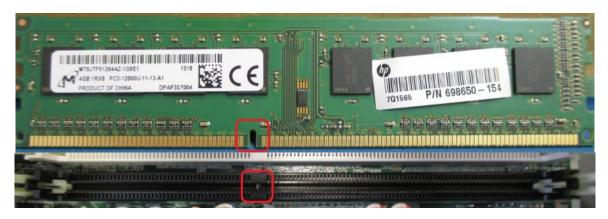
3) Install the replacement RAM into the notched RAM slot and push down on the sides of the RAM to lock into place.
