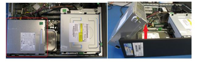
2) Remove 6 pin keyed power connector, P2, from PWRCMD connector as shown below.
