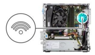
• Remove the retention screw, shield, and antenna connections as shown below, then slide the WLAN module out of the socket.
