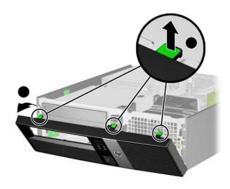
To install the new front bezel, reverse the removal procedure.
