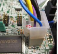
4) Remove the 4 pin lock tab connector, P3, from the PWRCPU connector and remove the wires from the cable holder on the fan duct connected to the CPU heat sink.
