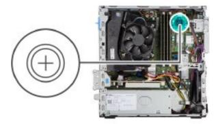
• Press the release tab and lift out the coin battery as shown below.
