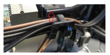
5) Slide the base of the power supply towards the inside of the computer.
