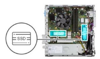
1. Remove the screw (M2x3) that secures the solid-state drive to the system board.
