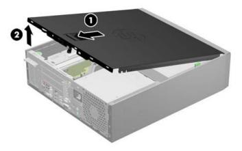
To install the computer cover, reverse the removal procedure.
