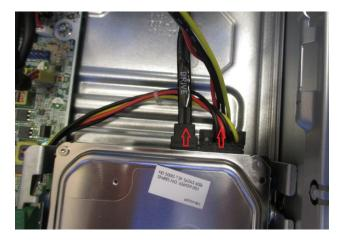
3) Push down release tab on side of hard drive guides to release the tab lock on the hard drive.
