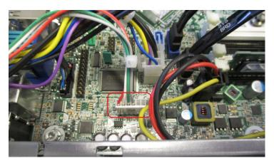
3) Remove the 6 pin lock tab power connector, P1, from the PWR connector.
