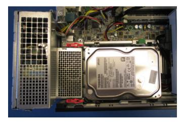
6) Lift the power supply up out of the power supply guides.
