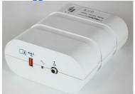
XScribe Front End is connected to the ECG A USB connector on the module front. One analog output connection is also on the front.
