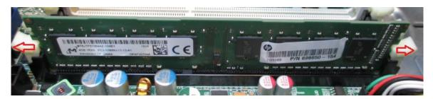
2) Take note on notch on RAM stick when installing replacement RAM.
