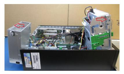
2) Remove both the SATA cable and power connector from the back of the hard drive.
