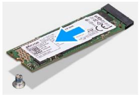
2. Slide at an angle to lift and remove the solid-state drive from its connector on the system board.
