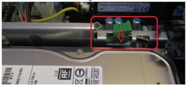
4) Slide the hard drive toward the inside of the computer and lift the hard drive out of the guides.
