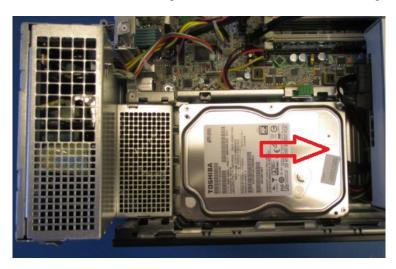
5) Remove the side screws from the old hard drive and put the screws onto the replacement hard drive.
